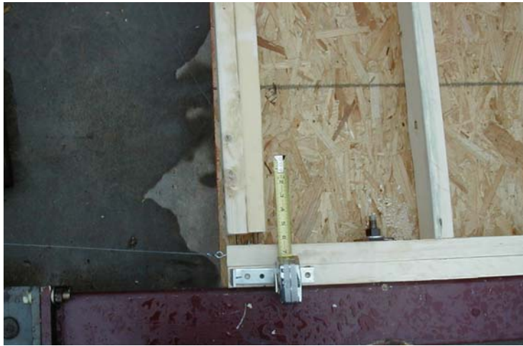
Figure 15: End stud separation at the top of the wall specimen (OSB)
