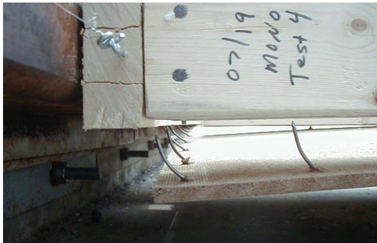
Figure 18: Nail pullout along bottom plate (hardboard)
