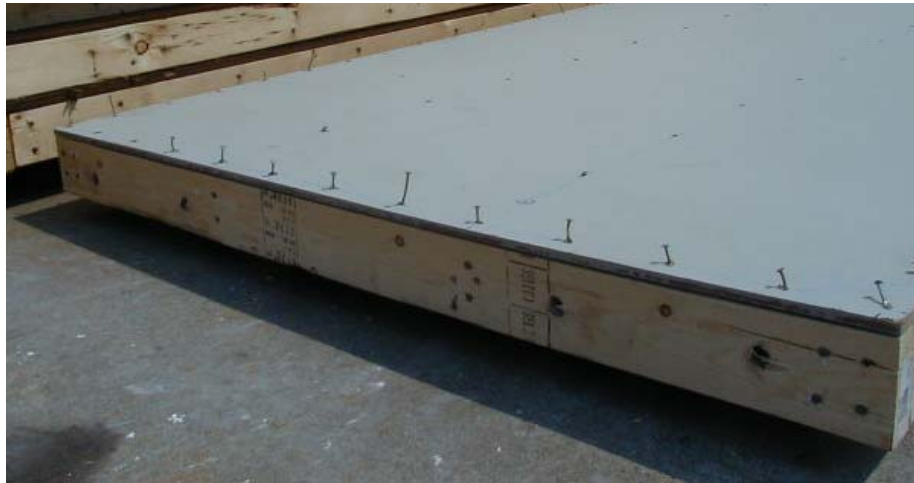
Figure 19: Nail pullout in hardboard panels
