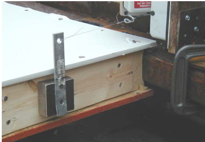
Figure 25: Racking displacement of sheathing panels
