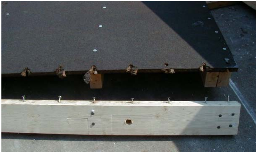
Figure 57: Nail pull through exclusively on bottom plate (fiberboard)
