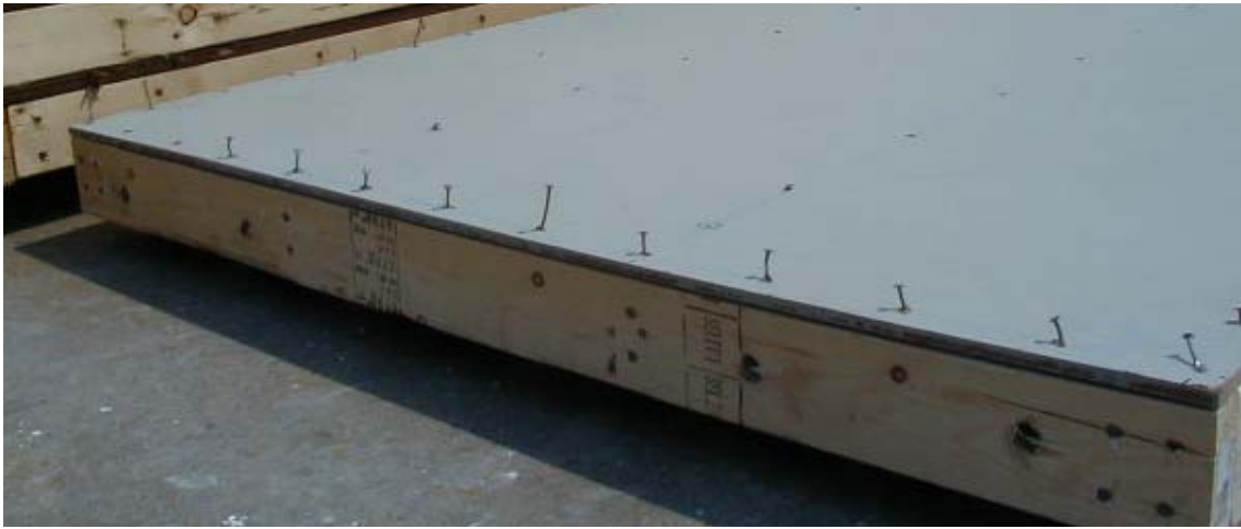
Figure 43: Nail pullout in hardboard panels
