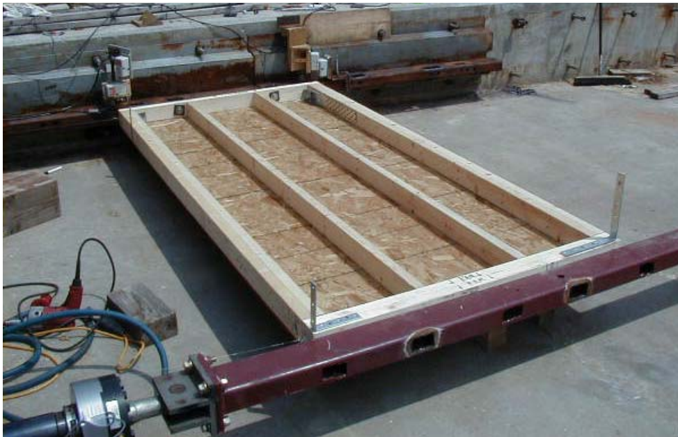
Figure 5: Test Setup with wall in-place
